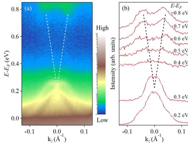
Fig. 1(a) Time-integrated Tr-ARPES image recorded around  $\bar{\Gamma}$  point of the SnTe (111) surface. (b) MDC plots at different binding energies extracted from (a)
