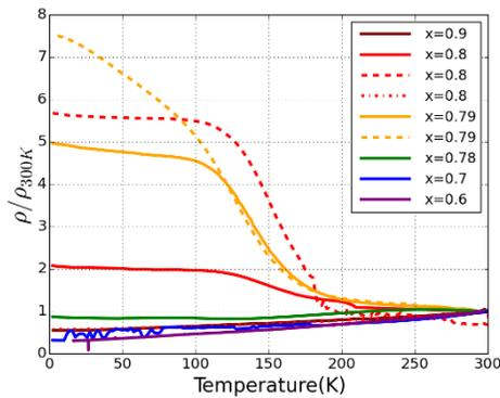
Fig. 1 Temperature dependence of resistivity measured for  $\text{Pb}(\text{Bi}_{1-x}\text{Sb}_x)\text{Te}_4$ .
