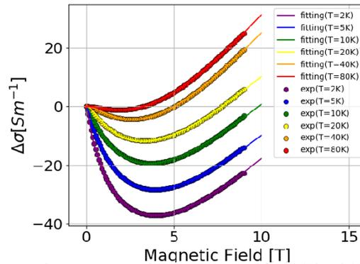
Fig.2 Magnetoconductance measured for  $\text{Pb}(\text{Bi}_{1-x}\text{Sb}_x)\text{Te}_4$  ( $x=0.79$ ), together with fitting curves.
