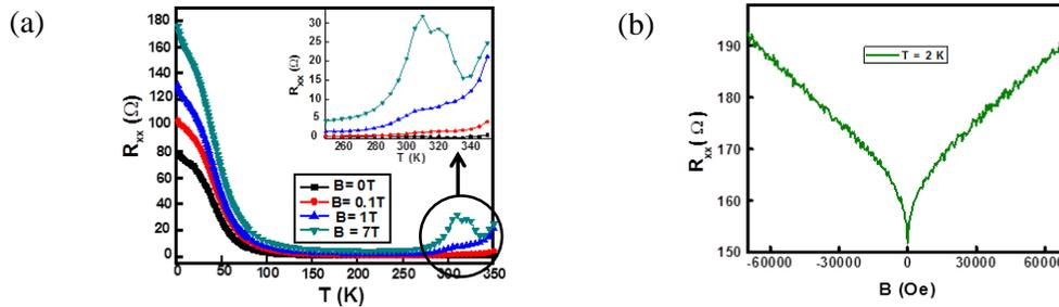
Fig.1. (a) Shows the  $R_{xx}$  variation with temperature in the range  $2 \text{ K} \leq T \leq 350 \text{ K}$  with magnetic field. (b) Shows the magneto-resistance behavior at 2 K with clear weak antilocalization effect is observed at zero magnetic field.
