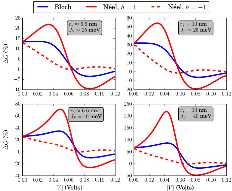
Figure : Relative change in conductance when a skyrmion is present with respect to the ferromagnetic texture
